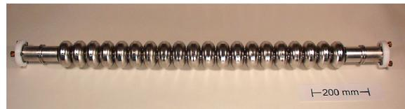
Figure 2: 20-cell niobium cavity.
