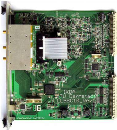
Figure 4: FPGA board containing the RF module and the baseband signal processing components.
