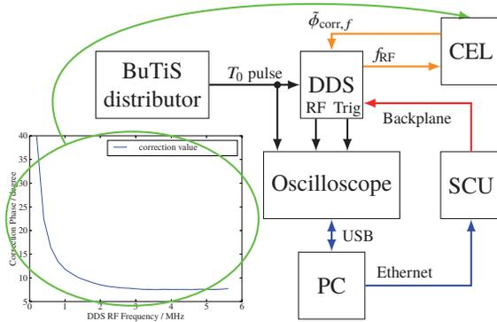
Figure 3: Measurement setup layout.
