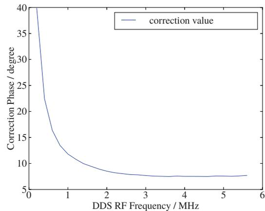
Figure 5: Example for a DDS module phase response measured with respect to BuTiS  $T_0$  pulse.
