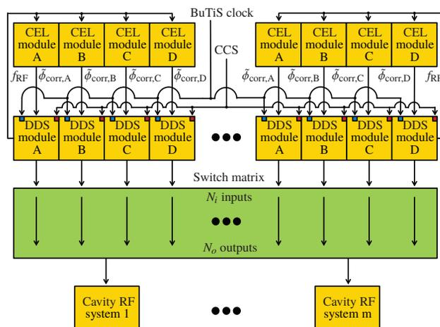
Figure 1: Routing of Group-DDS signals to cavity systems.
