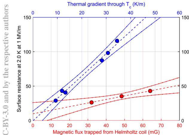
Figure 2: Measurements of the increase in residual resistance as a function of the applied thermal gradient (in blue) and trapped ambient magnetic field (in red) during the cool-down through  $T_c$ .
