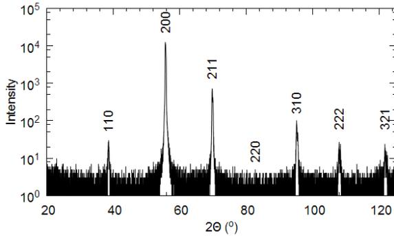
Figure 2: XRD pattern of a virgin Nb sample.
