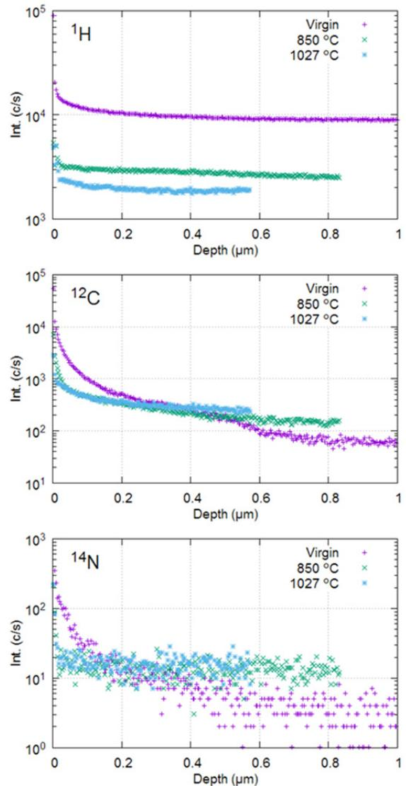
Figure 4: Comparison of the SIMS depth profiles for hydrogen (top), carbon (middle) and nitrogen (bottom) of the virgin and heat treated samples.
