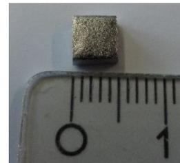
Figure 1: Niobium test samples cut from high quality Nb sheet. Typical sample size was 5x5x2.7 mm<sup>3</sup>.
