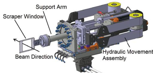
Figure 1: CAD illustration displaying the design of the scraper in ELENA.
