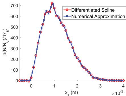
Figure 4: Comparison of a probability distribution obtained using a polynomial spline and simple numerical method.
