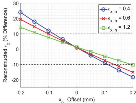
Figure 5: Effects of a closed orbit offset between positive and negative scraper scans on the reconstructed value of the horizontal rms emittance.
