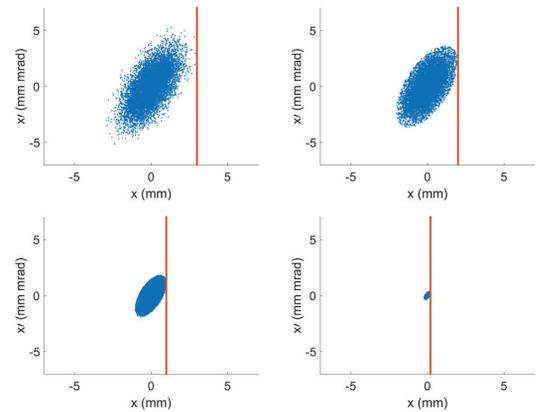
Figure 3: Transverse horizontal phase space of the antiproton beam during various stages of the simulated scraping process. The scraper blade is represented by the vertical red line.
