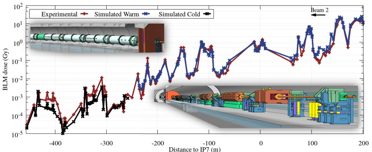
Figure 1: Simulated and measured BLM signals for the 2015 proton CQT at 6.5 TeV. Renderings of the IR7 and dispersion suppressor geometry models in FLUKA are shown in bottom right and top left corners, respectively. The beam direction is from the right to the left. The beam 2 primary collimators are located at around 200 m from the IP.
