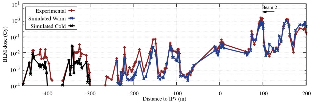
Figure 2: Cumulative BLM signals of the 2015 6.37 ZTeV Pb Ion CQT, Experimental vs Simulated
