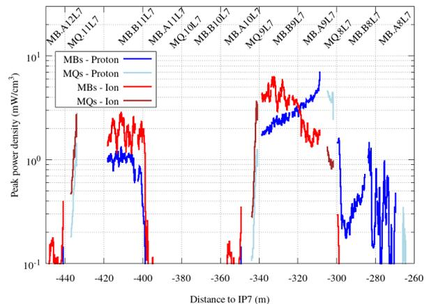
Figure 3: Simulated peak power density profile in the IR7 SC coils at the peak loss rate of the 2015 CQT for 6.5 TeV proton and 6.37 ZTeV Pb Ion
