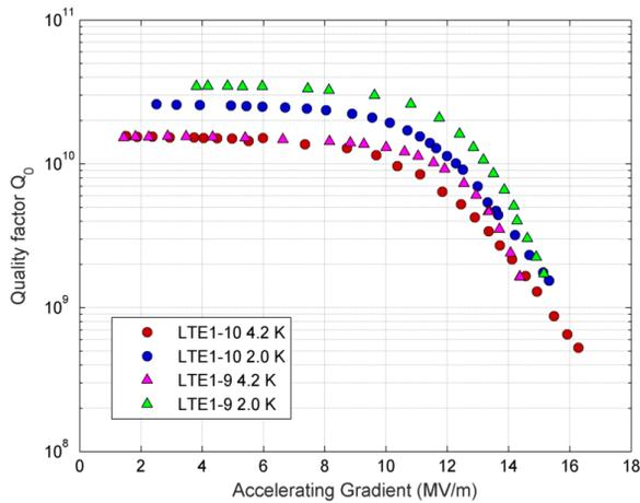
Figure 4: Quality factor vs. Accelerating field at 2.0 K and 4.2 K bath temperature for two cavities that received coating recipes that omitted the annealing stage.
