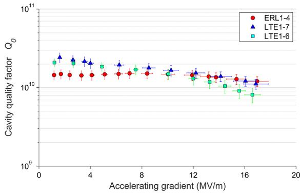
Figure 2: Quality factor vs. Accelerating field at 4.2 K bath temperature for three of the best cavity performances on the Nb<sub>3</sub>Sn program.
