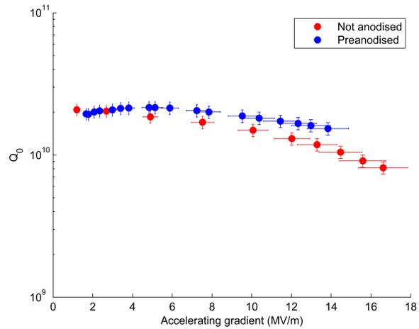
Figure 3: Quality factor vs. Accelerating gradient at 4.2 K bath temperature for a cavity having no anodisation before coating (red) and with pre-anodisation to 30 V before coating.
