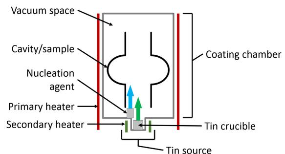
Figure 1: A simplified diagram of the Nb<sub>3</sub>Sn coating furnace.
