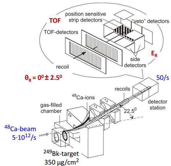
Figure 3: Kinematic recoil separator used for synthesis of SHE. The recoil products emitted from the target continue to move in hydrogen medium at a pressure of about 1 torr. Separation of reaction products occurs in a magnetic field. The distance from the target to the focal detectors is 4 m; the time of flight this distance by the heavy nucleus is about 1  $\mu\text{s}$ .
