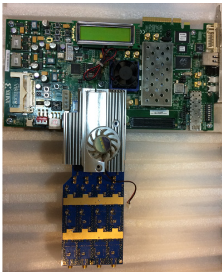
Figure 2: The overall hardware implemented design of BPM system.
