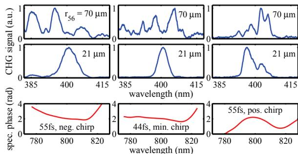
Figure 4: Spectral phase of 800-nm seed pulses (bottom) and CHG spectra at the second harmonic normalized to their maximum with the chicane set to  $r_{56} = 21 \mu\text{m}$  (center) and  $70 \mu\text{m}$  (top). The measurements were performed with three different settings of the laser compressor. From left to right: negative chirp, shortest pulse, positive chirp.
