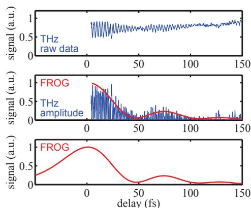
Figure 6: A high-cost low-resolution autocorrelator [14] for CHG seed pulses. A twofold energy modulation of the same electrons in two undulators is indicated by a periodic variation of the coherent THz signal (top). The amplitude of the variation (center) resembles the FROG result (bottom).
