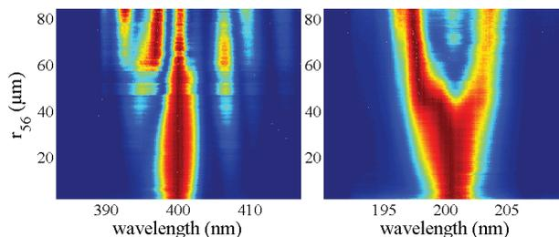
Figure 5: Sequence of 600 single-shot spectra of CHG radiation under slow variation of the chicane strength  $r_{56}$  while seeding with 800-nm (left) and 400-nm (right) laser pulses.
