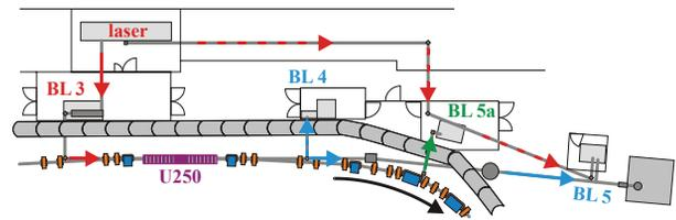
Figure 3: The short-pulse facility at DELTA comprising a laser system, a beamline (BL 3) sending seed pulses to the undulator U250, a diagnostics beamline (BL 4), a soft-x-ray beamline (BL 5), and a THz beamline (BL 5a).
