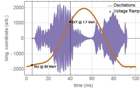
Figure 6: Longitudinal coupled bunch oscillations over the Booster cycle.
