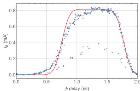
Figure 4: Current in Booster for varied injection phase.
