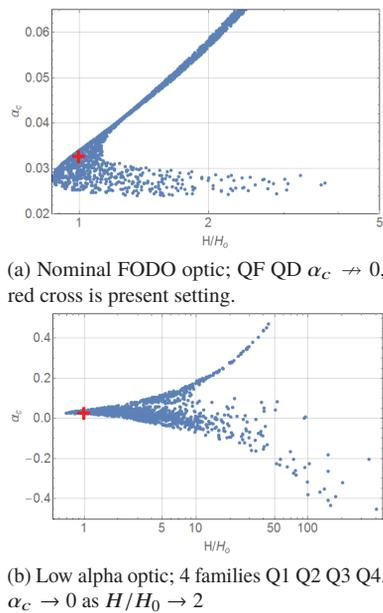
Figure 5: Towards low alpha optic in the Booster.
