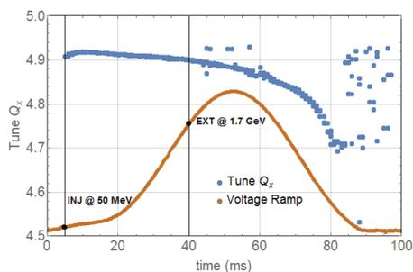
Figure 3: Horizontal tune over the 10 Hz Booster ramp. (for reference 5 ms injection, 40 ms extraction at 1.7 GeV)
