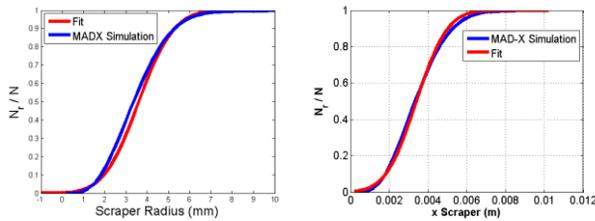
Figure 4: Cumulative beam distributions based on scraper position vs. particles remaining. The left figure shows the equation drawn against the data with  $\epsilon_x = 1.2$  mm mrad, and the right figure shows the resultant fit from the MATLAB fitting algorithm, resulting in  $\epsilon_x = 0.805$  mm mrad.
