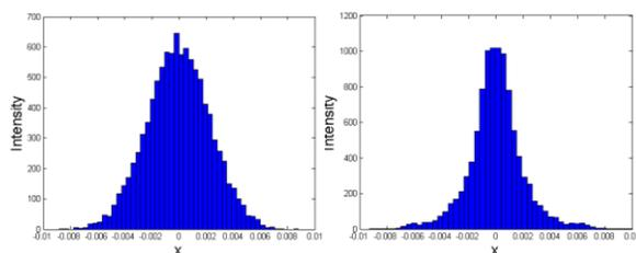
Figure 2: Gaussian and bi-Gaussian beam distributions.
