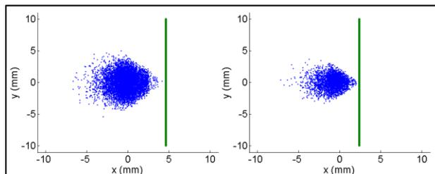
Figure 3: Transverse beam profile at  $x_s = 4.6$  mm and at  $x_s = 2.4$  mm. The blade position is represented by the green vertical line.
