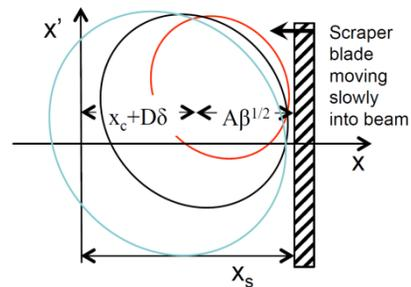
Figure 1: Schematic representation of a scraper; acceptance for a beam with zero momentum offset (black ellipse), with positive momentum offset (red ellipse) and with negative momentum offset (blue ellipse).
