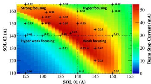
Figure 1: BS current and emittance measured as a function of SOL1&2 at the best working point found up to now.
