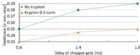
Figure 5: Emittance of the chopped beam of 100  $\mu$ s with and without Krypton gas for different delays of the chopper gate along the 2 ms source pulse (SOL1&2= 292&250 A).
