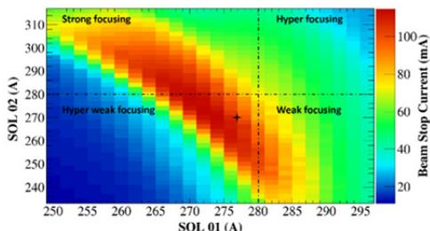
Figure 3: BS current measured as a function of SOL1 & SOL2 at 10% duty cycle; Highest current of 115 mA.
