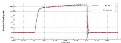
Figure 4: BS current of a chopped beam of 100  $\mu$ s (source pulse of 2 ms) with and without Krypton gas injection. (SOL1&2=292&250 A).
