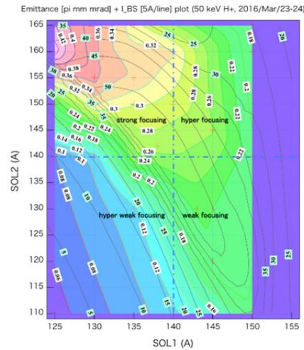
Figure 2: Emittance contour plot from the emittance values shown on Fig. 1 + BS current lines from data of Fig. 1.
