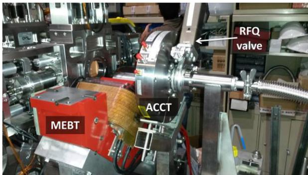
Figure 2: Assembly test of the ACCT.
