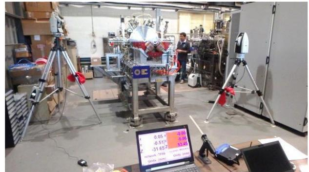
Figure 3: Two laser trackers and watch windows during MEBT alignment campaign.
