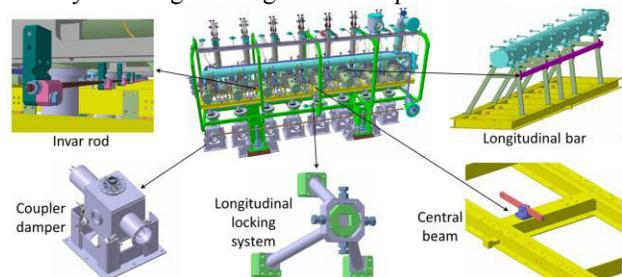
Figure 4: SRF Linac design optimisation following seismic analyses.
