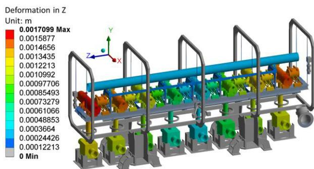
Figure 5: SRF Linac deformation after design optimization.
