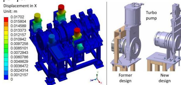
Figure 1: MEBT deformation from RS analysis and turbo pump design change.
