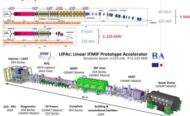
Figure 1: Above - Comparison of IFMIF accelerators and LIPAc, their 1.125 MW beam average power prototype accelerator, matched up to the 1st SRF linac at 9 MeV. Below - breakdown of the contribution for LIPAc.
