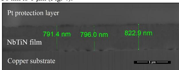
Figure 4: High magnification SEM of section of thin NbTiN film.
