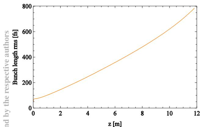
Figure 6: Simulation of bunch length growth over the length of VELA for a 1 pC bunch.
