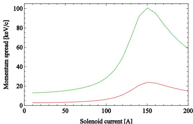
Figure 2: Simulated momentum spread at the sample as a function of solenoid current for a 1 pC beam (rms of distribution in red, full spread in green).
