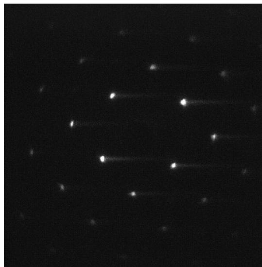
Figure 3: Single shot diffraction pattern from a single crystal Au(100) sample.
