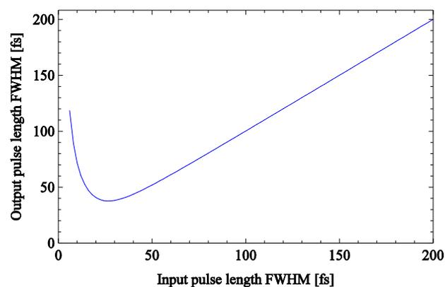
Figure 7: Laser pulse length after transport through 2 mm CaF<sub>2</sub>.
