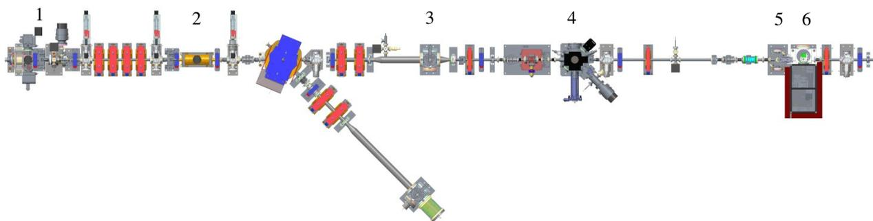
Figure 1: VELA schematic layout, showing: 1. Photoinjector gun, 2. Transverse deflecting cavity, 3. YAG screen used for bunch length measurements, 4. Sample chamber with independent stages for sample and beam shaping apertures, 5. Insertable Faraday cup, 6. Lanex screen used for imaging diffraction patterns.
