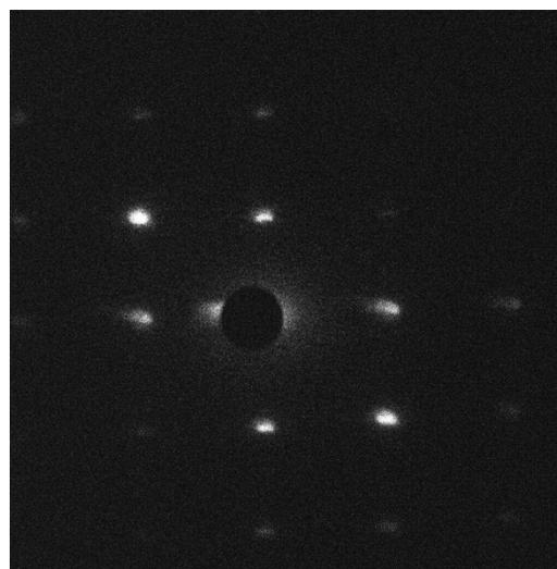
Figure 4: Single shot diffraction pattern from 100 nm thick Si(100).
