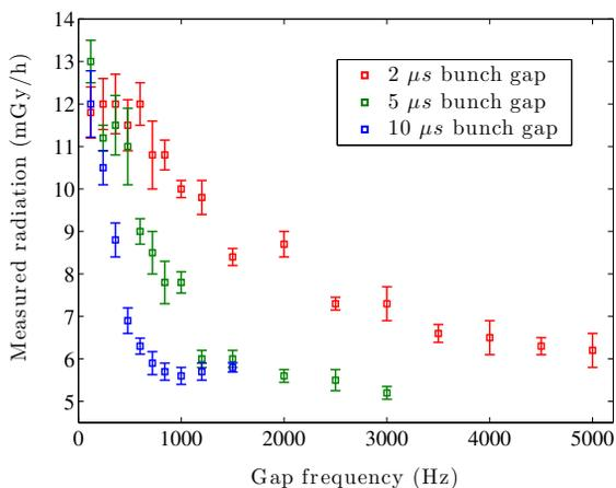
Figure 5: The number of trapped ions that reach the clearing electrode are reduced by increasing the frequency and duration of bunch gaps. The beam current was held fixed at 10 mA for this data, and the clearing electrode was turned off.
