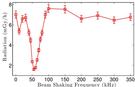
Figure 6: Shaking the beam at frequencies near the ion oscillation frequency eliminates the excess radiation caused by beam-ion interactions.
