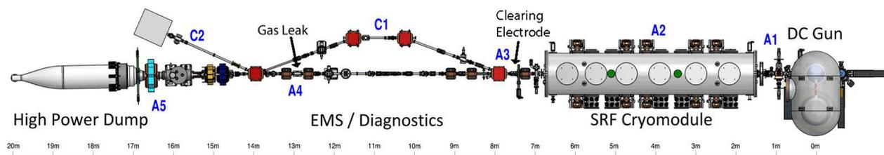
Figure 2: A schematic of the photoinjector that shows our experimental setup. Radiation measurements were taken using photomultiplier tubes at several locations between sections A3 and A4 (next to the beam pipe).
