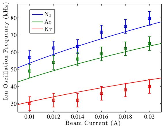
Figure 7: Resonance frequencies for various beam currents and ion species. The circles represent data points, while the lines indicate theoretical predictions [3].
