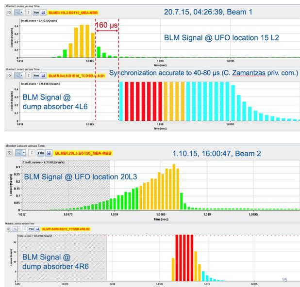
Figure 3: Screenshots of the BLM post-mortem analysis tool for a UFO event that dumped the beam without quench (top), and for a UFO event that caused a beam-induced quench (bottom).
