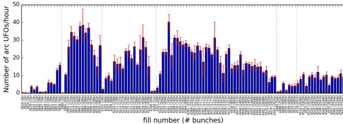
Figure 2: Rates of UFO events during physics production. The horizontal axis indicates the fill number and the number of bunches circulating per ring. The vertical dotted lines separate different operational periods: operation with less than 50 bunches/ring, with 50 ns beams, with 25 ns beams with up to 500 bunches, with 25 ns beams up to 1800 bunches, high-beta run with 100 ns spaced beams, with 25 ns beams up to 2244 bunches.
