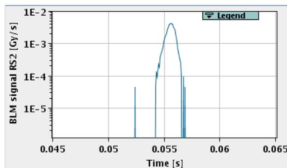
Figure 1: Typical signal shape of a UFO recorded by the capture buffer of the BLM system. RS2 stands for Running Sum 2, i.e. loss signals integrated over  $80 \mu\text{s}$ .
