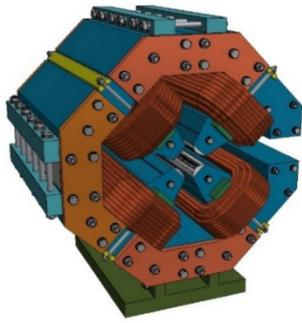
Figure 10: Perspective mechanical design of the SR quadrupole [7].
