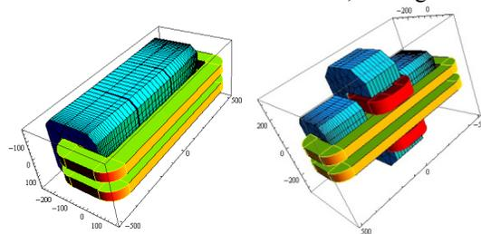
Figure 2: 3D design of the main (left) and high field inserted (right) SR dipole magnets[8].
