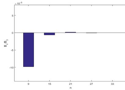
Figure 12: Normalized multipole errors at +13.5 mm.
