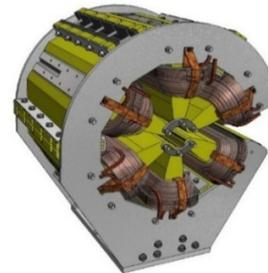
Figure 13: Perspective mechanical design of the SR sextupole [7].
