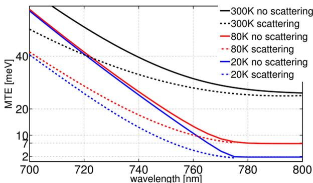
Figure 4: MTE at different temperatures (300K, 80K and 20K). The solid lines represent MTEs from no scattering [8]; The dotted lines show MTEs from simulation using scattering with 150nm thickness, reflection cathode.
