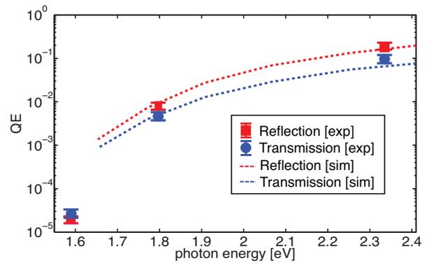
Figure 2: Quantum efficiency as a function of photon energy. The QE data (dot) at each wavelength are measured at 250 kV. The simulation QE is presented in the dotted line (the QE was scaled with a scaling coefficient.)
