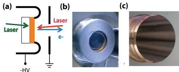
Figure 1: (a) A schematic for direction of light and photoelectrons: green arrow for transmission mode, red arrow for reflection mode. (b) a photocathode used in the experiment with a glass in the middle (c) typical photocathode (only reflection mode is allowed)
