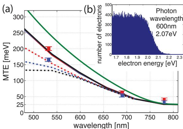
Figure 3: (a) MTE from Monte-Carlo simulations and experimental data (reflection (red dot) and transmission (blue dot)) as a function of laser wavelength at three different photocathode thicknesses: 150(red), 300(blue) and 500(black) nm. Dotted lines represent the transmission mode. The green line is calculated with the model from Ref. [8]. (b) A histogram of excited electrons above  $E_w$  following a FD distribution at room temperature.
