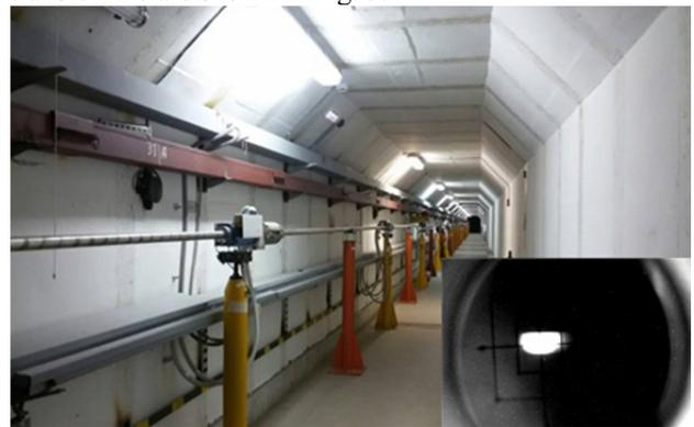
Figure 5: VEPP-5 – VEPP-2000 beam transfer line (right down corner – view of the beam at the phosphor screen at the end of transfer line).
