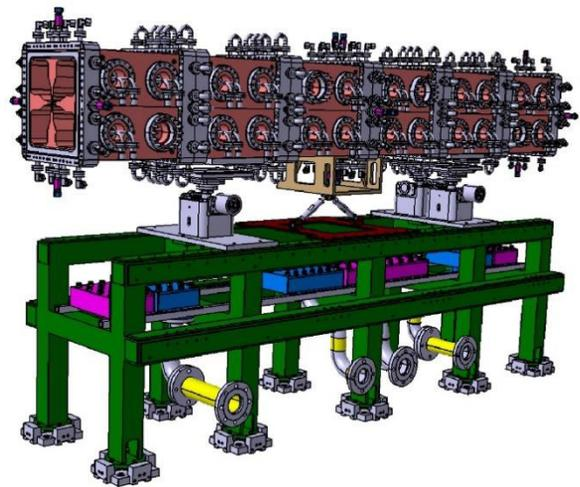
Figure 2: RFQ central SuperModule.
