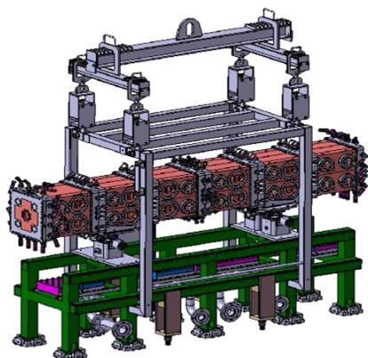
Figure 3: RFQ SuperModule lifting tool.
