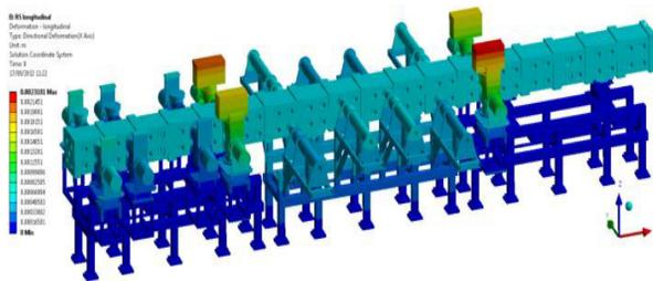
Figure 5: RS analysis longitudinal deformation.
