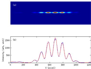
Figure 2: CCD image and horizontal intensity profile.
