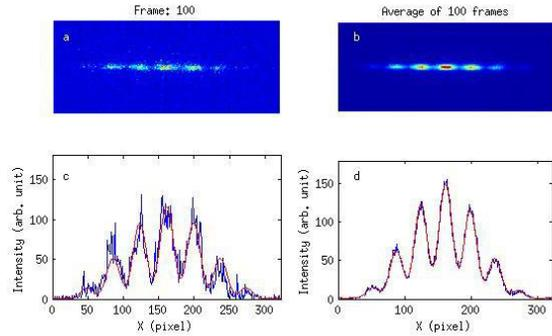
Figure 3: A single-shot image and its horizontal profile (left) and the averaged image over 100 frames (right).
