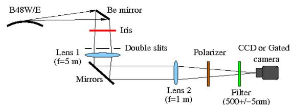
Figure 1: Schematic layout of the setup.
