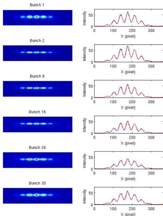
Figure 5: Interference pattern of 6 different bunches in a 30 bunch positron bunch train.
