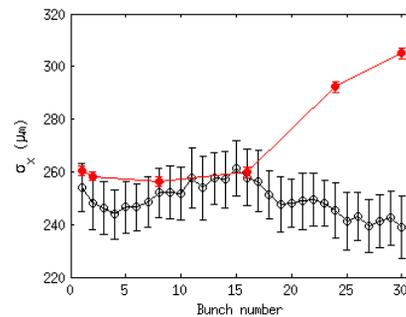
Figure 6: Horizontal beam size of a 30 bunch train of positrons (red) and electrons (black).
