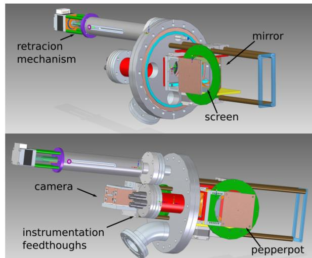
Figure 3: Emittance meter design details.
