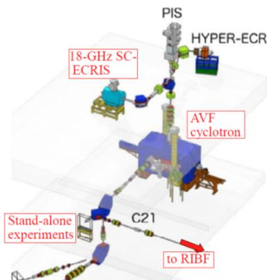
Figure 1: RIBF injector complex including the 18 GHz SC-ECRIS.
