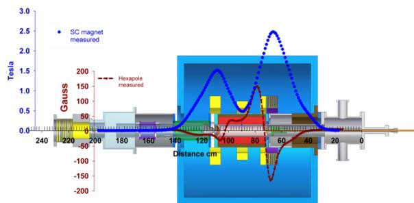
Figure 2: Illustration of the magnetic field distribution.
