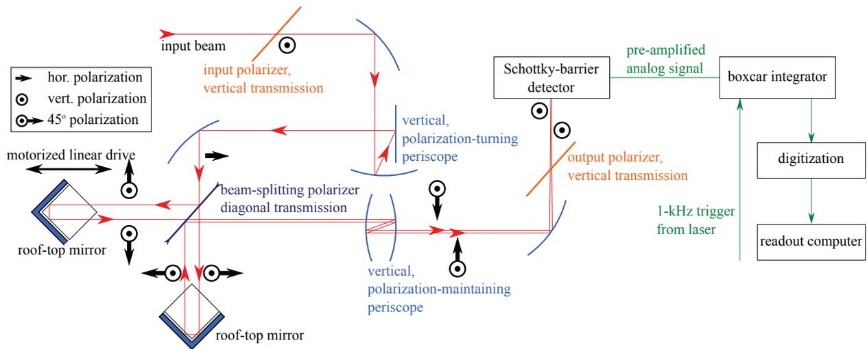
Figure 3: Setup of the polarizing spectrometer commissioned at the short-pulse facility (see text for details).
