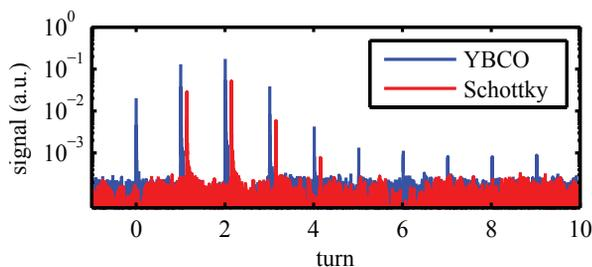
Figure 2: Signals of the YBCO and Schottky-barrier detector several revolutions after the laser electron interaction. For better visibility the signal of the Schottky diode is shifted by 30 ns.
