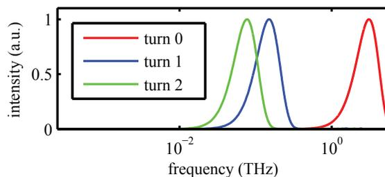
Figure 1: Simulated coherent THz spectra from turn 0 to turn 2 normalized to peak intensity (see text for details). The simulation is based on the code THzSMe [7, 8].
