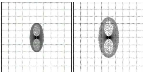
Figure 6: The probe electron beam images on the observation screen for 2 (left) and 1 ps (right) long bunch; grid size is 2 mm.
