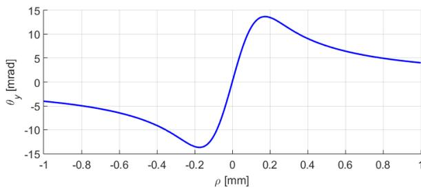
Figure 2: Deflection angle  $\theta_y$  as a function of the impact parameter  $\rho$  for 1 ps bunch RMS length and 100  $\mu\text{m}$  transverse RMS size.
