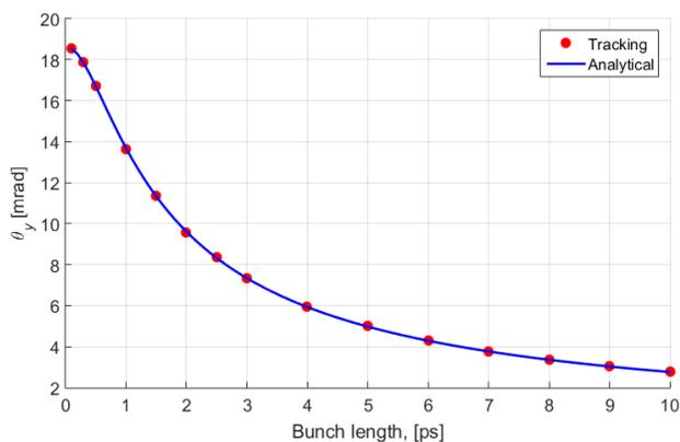
Figure 5: Maximal vertical deflection angle as a function of the bunch length according to Eq. 1 – blue curve and according to the particle tracking simulation – red dots.
