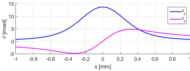
Figure 1: Deflection angles  $\theta_y$  and  $\theta_z$  as a function of the electron position inside the probe beam.
