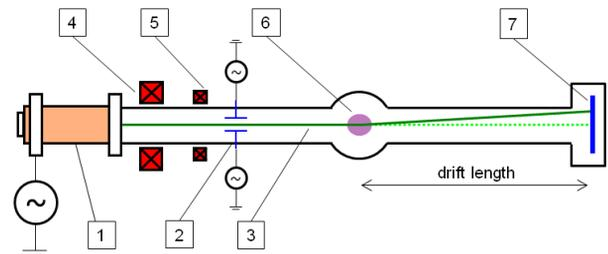
Figure 4: Diagnostic layout: 1 – electron gun, 2 – horizontal deflecting plates, 3 – probe electron beam, 4 – focusing solenoid, 5 – magnetic correctors, 6 – electron bunch, 7 – observation screen.
