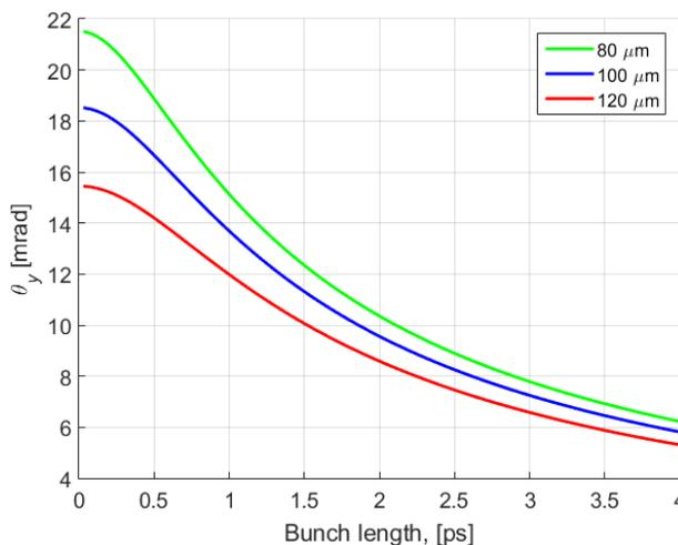
Figure 3: Maximal vertical deflection angle  $\theta_y$  of the probe electrons as a function of the bunch length for three transverse bunch sizes 80, 100 and 120  $\mu\text{m}$ .
