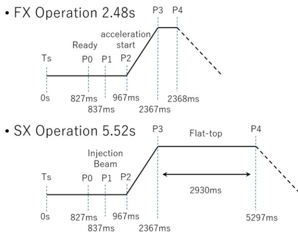
Figure 1: MR operation cycle of the two modes.
