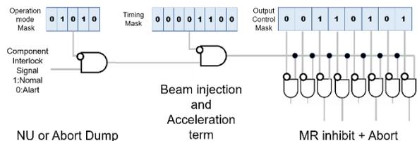
Figure 7: MR-MPS signal output logic.
