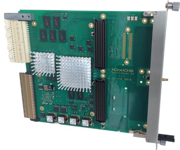
Figure 1: IOxOS IFC1410 MicroTCA board.
