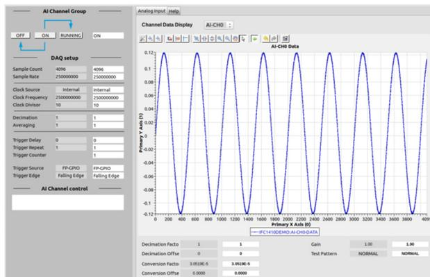
Figure 3: User interface running in CSS plotting analog signals acquired with IFC1410.
