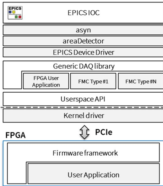
Figure 2: Software stacks of MicroTCA integration at ESS.
