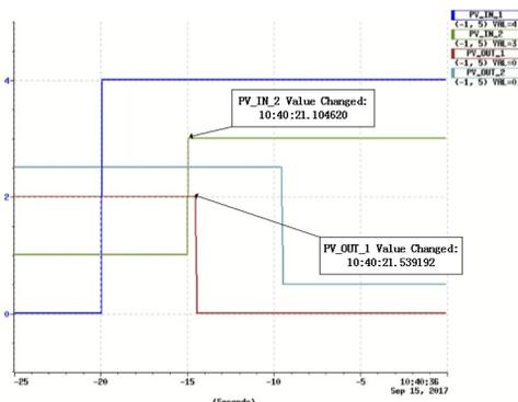
Figure 6: Execution Result of Soft Interlock System.
