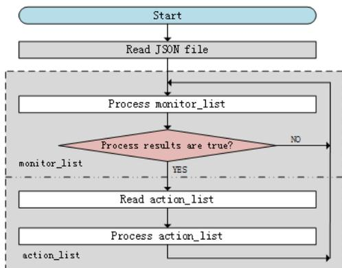
Figure 5: Flow chart of Software Interlock System.
