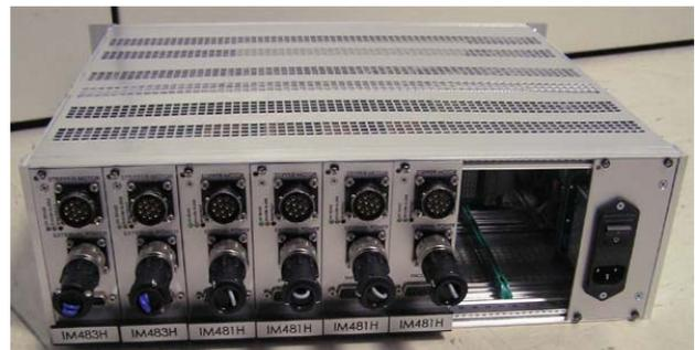
Figure 2: YAMS chassis (rear view).
