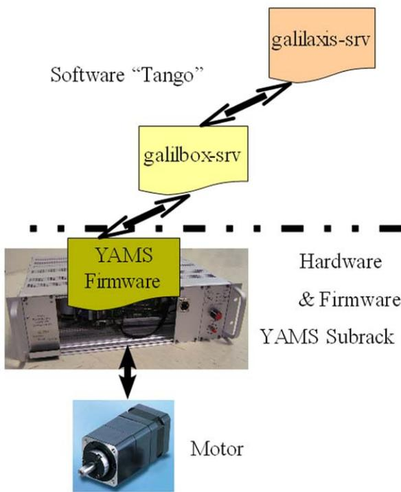
Figure 5: Hardware/Software Architecture.
