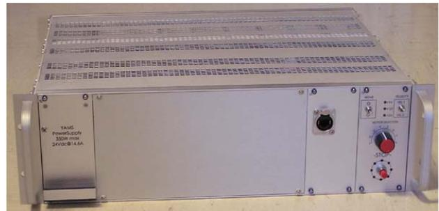
Figure 1: YAMS chassis (front view).
