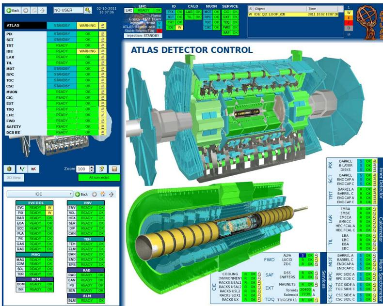
Figure 3: Operator interface (FSM Screen) showing the detector in *STANDBY* configuration during LHC ramp-up. The top hierarchy level object is shown together with its children objects (top left) and the associated main panel (bottom right). The UI allows the navigation to any FSM object and associated panel within the whole ATLAS DCS hierarchy. On the top right, a list of objects with non-OK Status allow shortcut navigation to problems.
