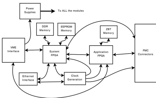
Figure 2: Block diagram of CERN's VME FMC carrier.
