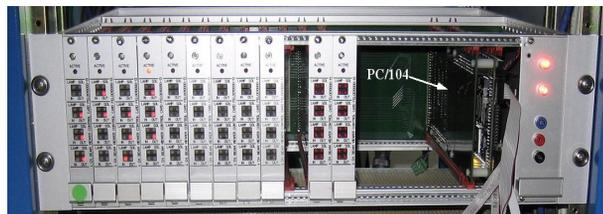
Figure 2: The new FEL beam viewer control crate.
