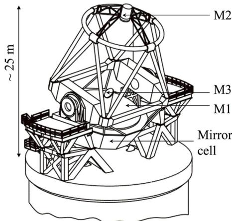
Figure 2: Sketch of a VLT Unit Telescope. The three principal mirrors are indicated.
