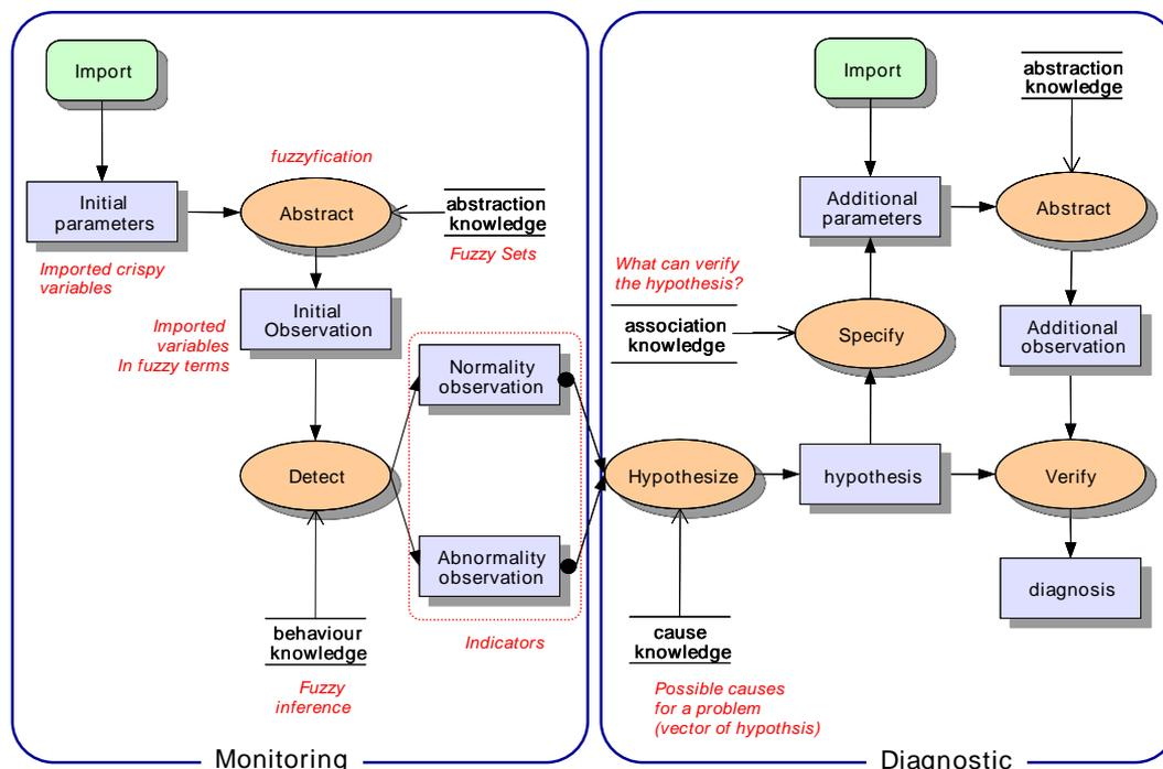
Fig. 2 CommonKADS Knowledge Model Template for Monitoring and Diagnostic analytic tasks. Rounded-squares are transfer functions, ovals are Inferences, and squares are domain concepts.
