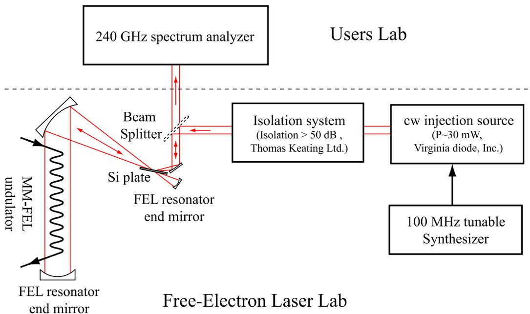
Figure 3: Schematic of the injection locking system for the UCSB MM-FEL. The injection source, the isolator and a tunable 100 MHz synthesizer are located in free-electron laser lab. Output radiation is sent to the users lab through vacuum optical transport system.
