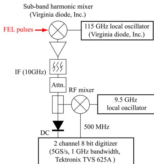
Figure 4: Schematic illustration of the 240 GHz spectrum analyzer.
