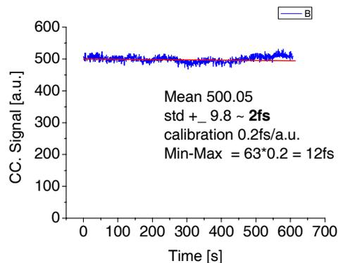
Figure 7. Typical cross-correlation signal by the jitter-measurement
