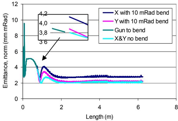
Figure 2: Emittance (normalised) (1 nC, 3.7 MeV, 10ps). off axis compensation (10mR) at 0.75 m and linac from 1m.
