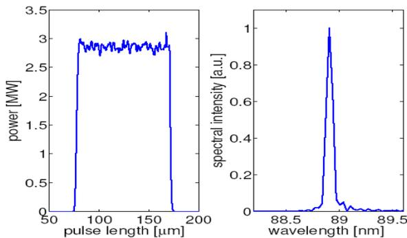
Figure 6: Temporal and spectral power distributions of FEL pulse at exit of radiator.
