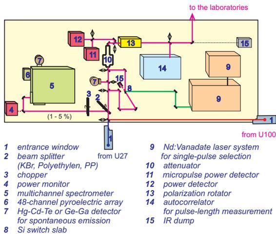
Figure 3: The IR diagnostic table. [4]
