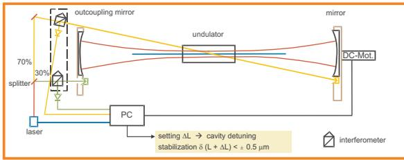
Figure 2: Schematic view of the resonator length control and stabilization system. Its time constant is 1 Hz and hence fast in comparison to the thermal time constant of the resonator.
