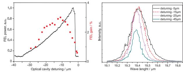
Figure 4: The saturation power (line) and the FEL single-pass gain (dots) (left panel) and the IR spectra (right panel) shown for varying optical cavity detuning.
