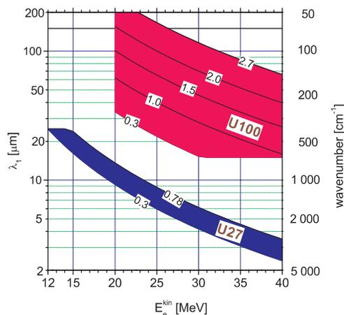
Figure 1: Wavelength ranges  $\lambda_1$  of the existing U27 and the planned U100 undulator of ELBE as a function of the kinetic electron energy  $E_e^{kin}$  calculated for the indicated values of the undulator parameter  $K_{rms}$ .
