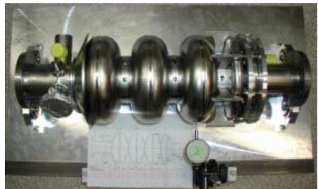
Figure 2: Photograph of the 3 1/2 cell Nb cavity.
