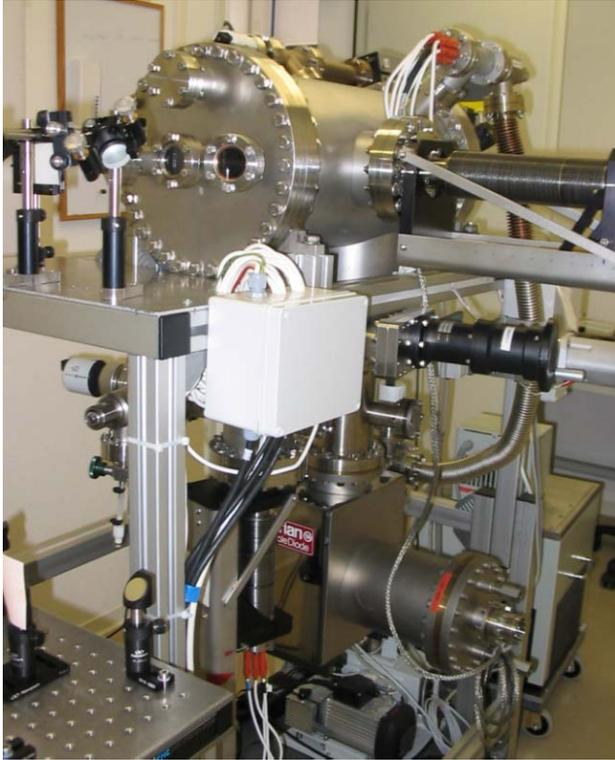
Figure 4: Photocathode preparation chamber.
