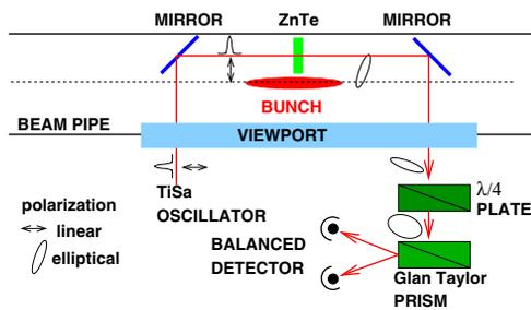
Figure 5: Setup of the bunch length monitor system with Electro-Optical Sampling. The arrows and ellipses indicate the orientation of the polarization when the electron beam moves in the vicinity of the crystal.
