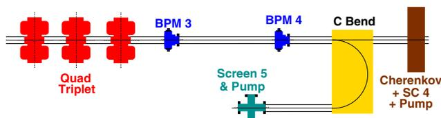
Figure 6: Setup of the energy and energy spread measurement.
