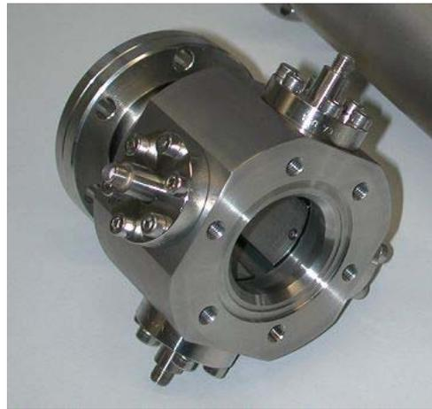
Figure 3: Short stripline BPM. The BPM is 85 mm long, the inner diameter of the beam pipe clearance is 40 mm.
