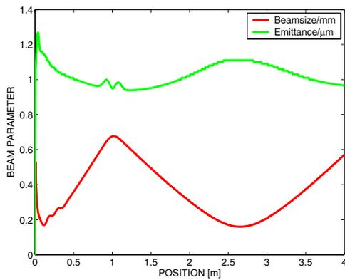
Figure 1: Propagation of beamsize and emittance for the ELBE mode with the modified emittance compensation scheme with input parameters like bunch length of 5 ps fwhm and with thermal emittance of  $0.7 \mu\text{m}$ . The peak magnetic flux density is 230 mT at 1.0 m distance from the cathode. Clearly visible the working point at 2.66 m.
