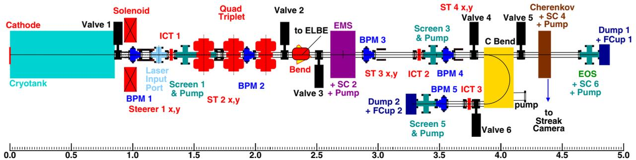
Figure 2: Diagnostics beamline overview including dipole magnet for the transfer to ELBE.
