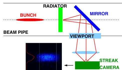
Figure 4: Setup of the bunch length monitor system with the Cherenkov radiator aerogel, the thickness of aerogel is 6 mm resulting in a time resolution of 0.4 ps.
