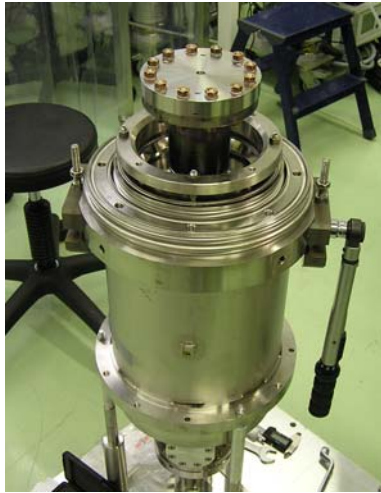
Fig. 12: Photograph of the He tank and cavity.
