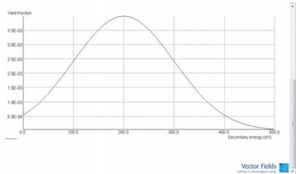
Figure 4: Gaussian secondary emission fraction used for simulations.
