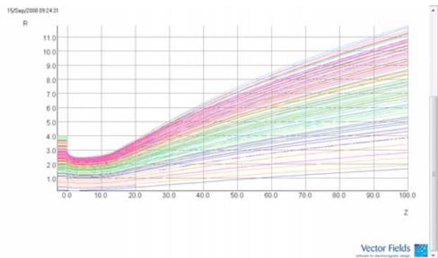
Figure 9: Ion beam without neutralization, note vertical scale.
