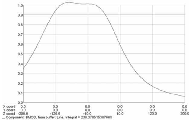
Figure 5: On-axis magnetic flux density.
