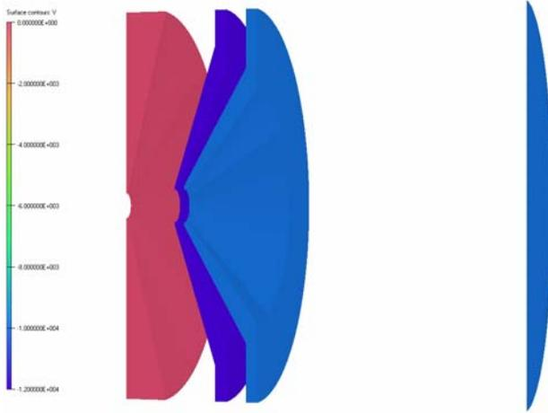
Figure 3: Boundary conditions, 0 V, -12 kV, -10 kV.
