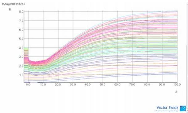
Figure 10: Ion beam with neutralization, note vertical scale.
