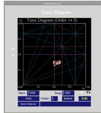
Figure 6: Tune evolution on tune diagram during energy ramping test run.
