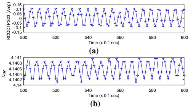
Figure 4: Tune variation due to 200 mA peak-to-peak sinusoidal wave applied to quadrupole trim (RCR1QDPS16).
