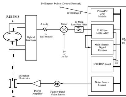
Figure 2: Functional block diagram of the digital receiver tune monitor and bunch-by-bunch current monitor.
