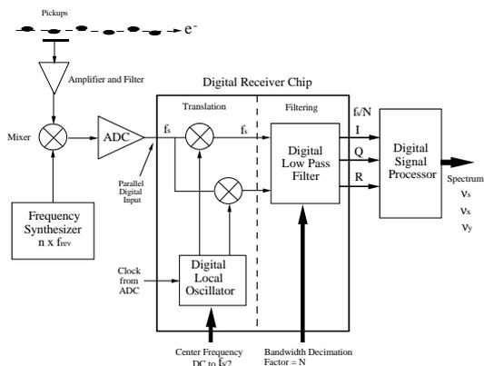
Figure 1: Functional block diagram of digital receiver
