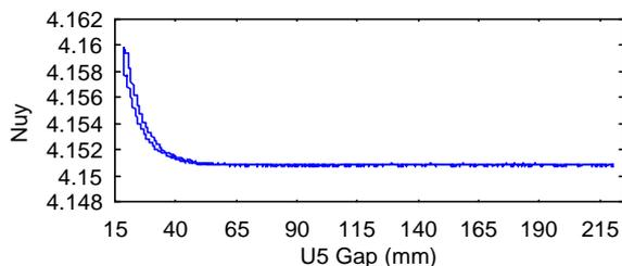
Figure 5: Vertical tune shift versus U5 gap.
