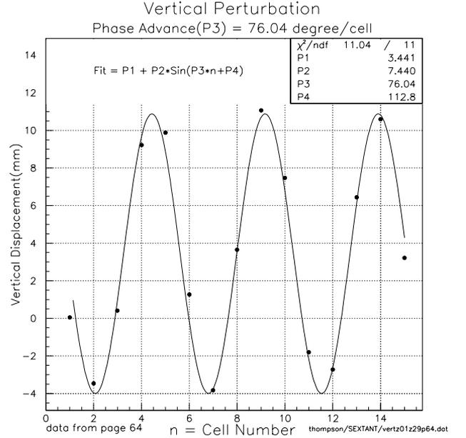
Figure 3: Measurement results of the FODO cell vertical phase advance.
