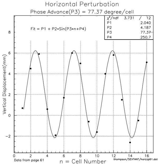
Figure 2: Measurement results of the FODO cell horizontal phase advance.
