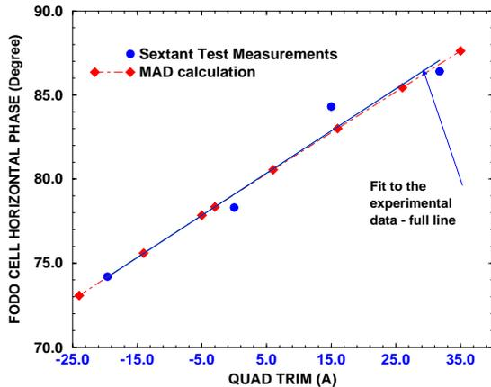
Figure 4: Dependence of horizontal phase advance per FODO cell on the quad *trim* current compared with the MAD results.
