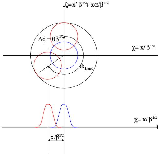
Figure 1: Beam profiles and dipole kicks presented in normalized phase space.
