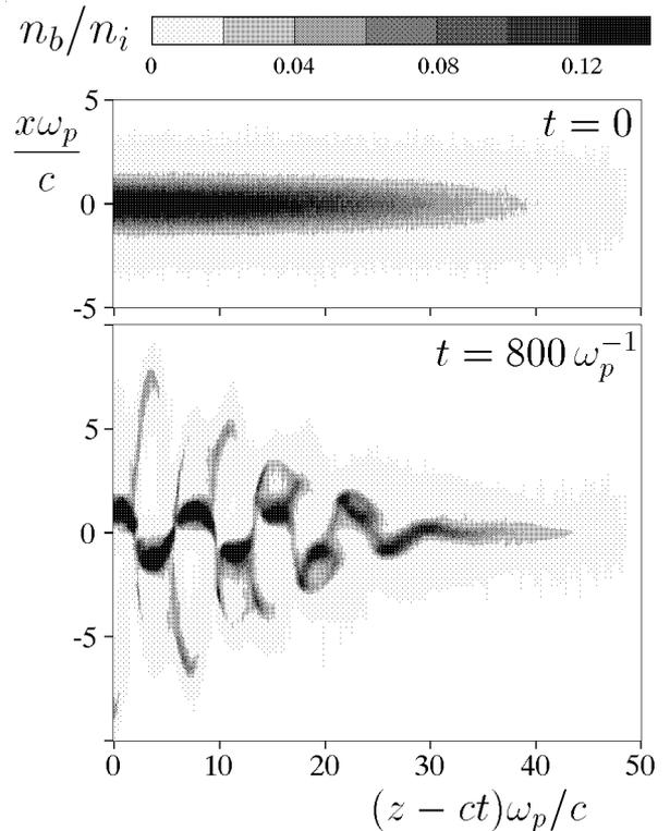
Figure 1: Destruction of the long beam by TTS instability. Plane geometry.
