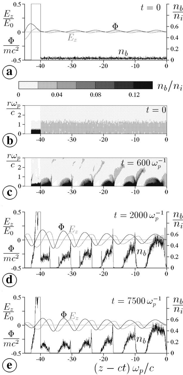
Figure 2: Self-modulation of the long axisymmetric beam with a sharp front.
