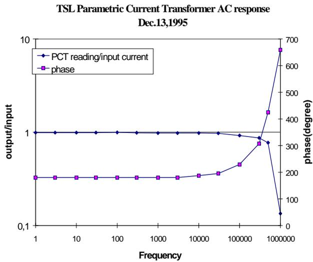
Fig. 4. PCT frequency response.
