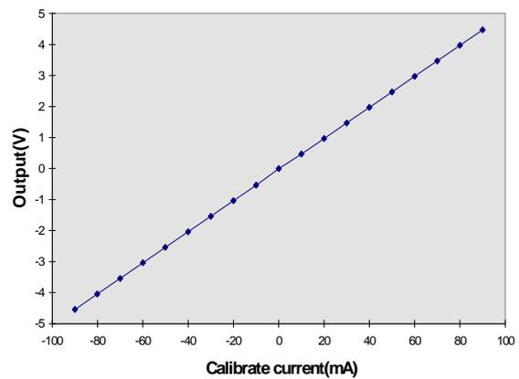
Fig. 2. Linearity calibration curve
