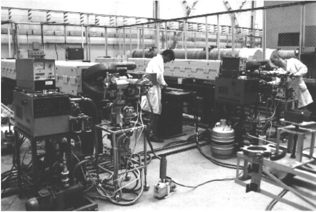
Figure 3: Assembling of the dipoles with the vacuum chambers.
