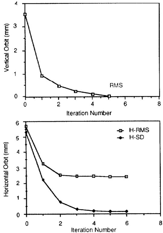
Fig. 7. Correction of the vertical and horizontal orbits, showing the average horizontal offset.
