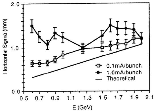
Fig. 6. Horizontal beam size measured by a photo diode array during the energy ramp, at 0.1 and 1.0 mA per bunch.
